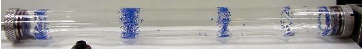
Figure 16. Band formation of particles due to capillarity. The fluid is glycerin with a density of 1.173 \text{ g/cm}^3 , a viscosity of 1490 \text{ cp} , and a surface tension of 41.46 \text{ mN/m} . The particles are polymer particles with a density of 1.034 \text{ g/cm}^3 and a diameter of 0.65 \text{ mm} . The filling level of the fluid is 10.5 \% and the particle concentration is 4.8\% . The rotating speed \Omega = 5.45 \text{ rpm} , \beta = 1.443 , average film thickness D_a = 0.753 \text{ mm} , minimum film thickness D_{min} = 0.605 \text{ mm} , D_{min}/d_p = 0.931 . Band formation 15 hours after beginning of rotation is shown in the figure.
