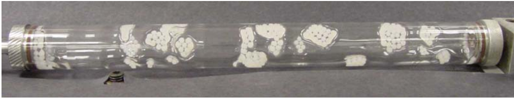
Figure 14. Clustering of particles due to capillarity. The fluid is glycerin with a density of 1.173 \text{ g/cm}^3 , a viscosity of 1490 \text{ cp} , and a surface tension of 41.46 \text{ mN/m} . The particles are white Nylon particles with a density of 1.170 \text{ g/cm}^3 and a diameter of 0.314 \text{ cm} . The filling level of the fluid is 8.2\% and the particle concentration is 54.2\% . The rotating speed \Omega=5.45 \text{ rpm} , \beta=1.127 , average film thickness D_a=0.585 \text{ mm} , minimum film thickness D_{\min}=0.526 \text{ mm} , D_{\min}/d_p=0.176 . Clusters of particles form about 5 minutes after starting of rotation. Bands form occasionally but are not stable.
